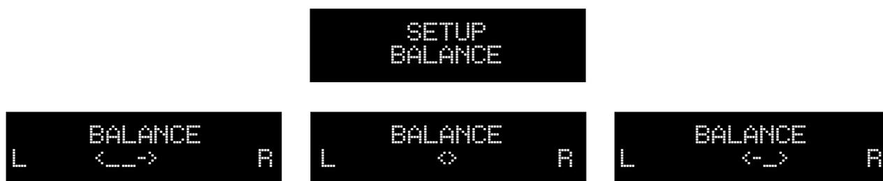
Left channel is increased with regards to right channel by rotating the encoder counter clockwise or by pushing the “arrow left” key on the remote control; right channel is increased with regards to left channel by rotating the encoder clockwise or pushing the “arrow right” key on the remote control.
